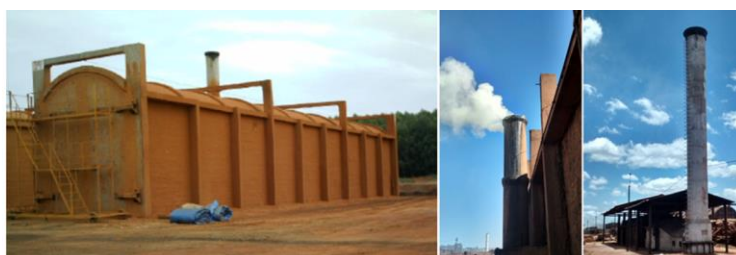
Figure 1. From left to right, charcoal rectangular kiln, kiln chimney, and gas burner
